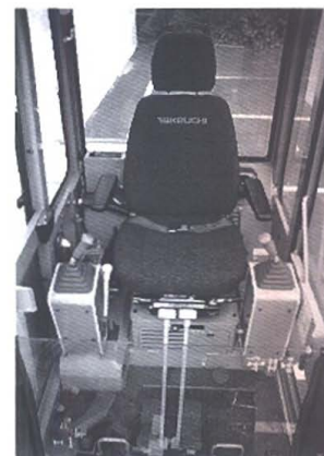
Feature packed operator's compartment with fully adjustable suspension seat, roll back front window, tinted glass, heater, defroster, windshield wiper/washer, AM/FM cassette radio, hand and foot operated travel levers and joystick servo controls.
